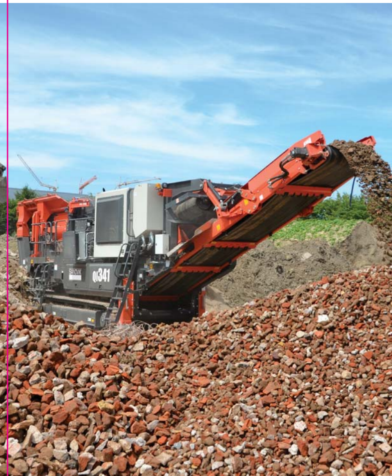
Featuring Sandvik's unique CI411 Prisec™ impact chamber (5 patents pending). The Prisec™ concept enables one base crusher to be configured as either a Primary or Secondary chamber whilst maintaining optimum crushing geometry.
